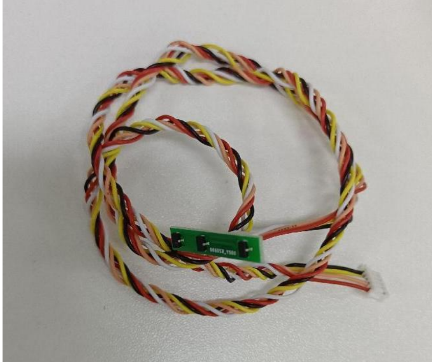
(Figure 6: Magnetic sensor (green chip) and magnetic sensor assembly line)
